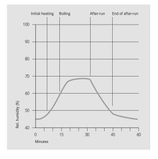
**Test** 30 min intensive boiling of 1.8 I water
