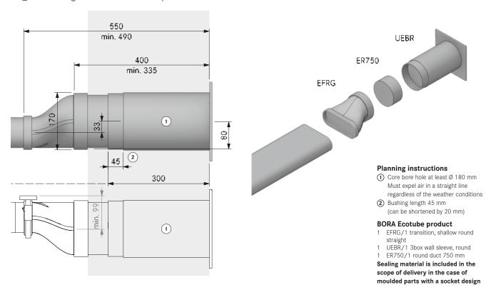
MP\_9068 ducting upright with transition piece EFR90 to wall sleeve UEBR
