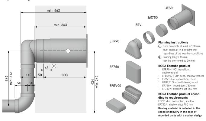
MP\_9066 ducting shallow with transition piece to wall sleeve UEBR
