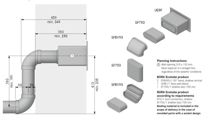
MP\_9062 ducting with S-bend wall sleeve UEBR
