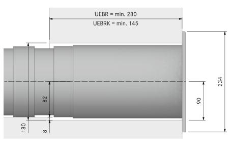
Please note that the wall sleeve has a protrusion on the lower end.
