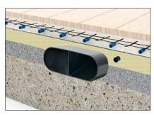
Shallow duct partially in the balancing layer and the reinforced floor screed
