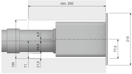
Please note that the wall sleeve has a protrusion on the lower end.
