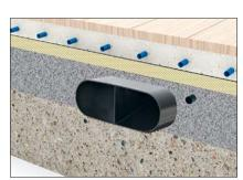
Shallow duct in the balancing layer (acc. to DIN 18560-2)
